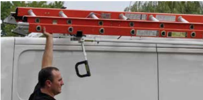
Lift ladder off the rear bracket.
